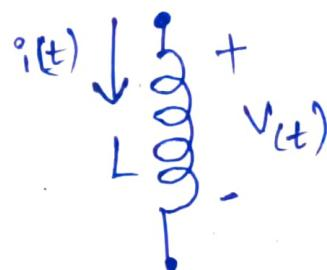
$$V_L(t) = \frac{d\phi}{dt} = \frac{dL_i}{dt} = -L \frac{di}{dt}$$
