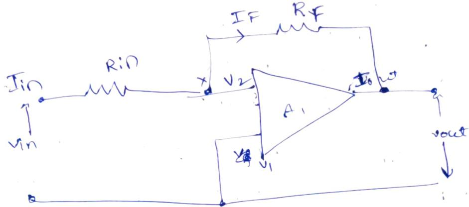
$$A_V = \frac{V_{out}}{V_{in}}$$
